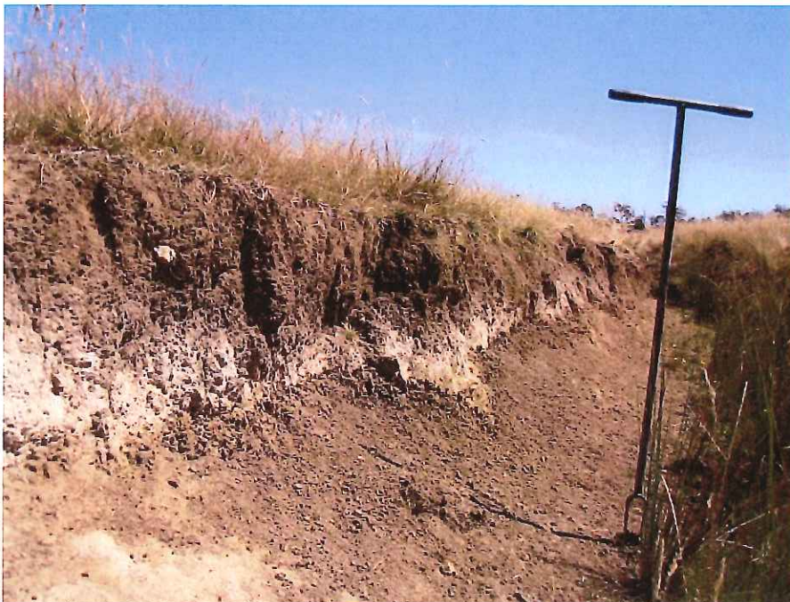
Photograph 6. Site 29. GDA 513822 5398249. Brumby soils in Quaternary alluvium, showing variable depth of sandy upper layers (pale layer and horizons above) over subsoil clay.
