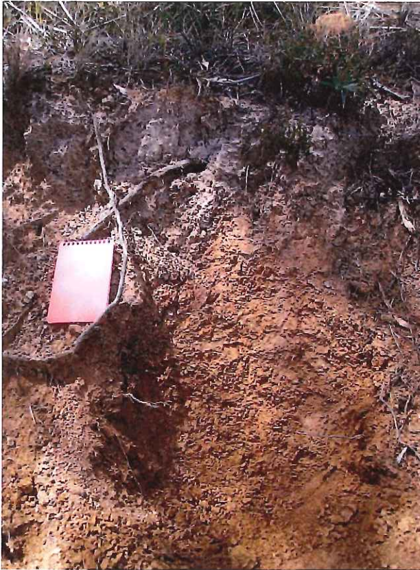
Photograph 3. Site 15. GDA 514572 5401313. Deep Eastfield soil in dolerite ( Ea ). The pale sandy upper horizons of the soil (probably aeolian) are very evident.
