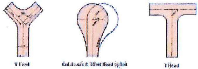
Figure 4 - Private Roadway Turning Head
