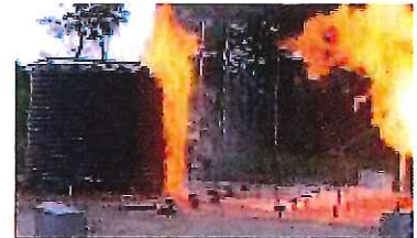
Figure 8 - Poly tanks NOT SUITABLE in bushfire areas
