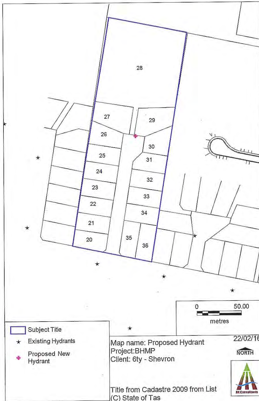
Figure 6: Proposed Fire Hydrant Location
