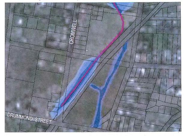
Figure 4.5 Model 3 - Proposed Subdivision Layout No. 2 Flood Plan
