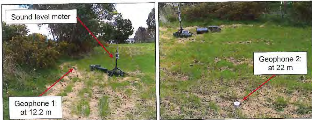
Figure 2 – Sound level and ground vibration meters located towards eastern boundary.
