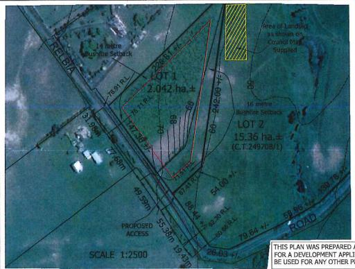
RELBIA ROAD CENTRELINE GRADES LENGTH, 31.98m, GRADE 3.8% LENGTH, 77.68m, GRADE 8.2% LENGTH, 49.59m, GRADE 8.3% LENGTH, 55.38m, GRADE 9.2% LENGTH, 19.43m, GRADE 8.4%
