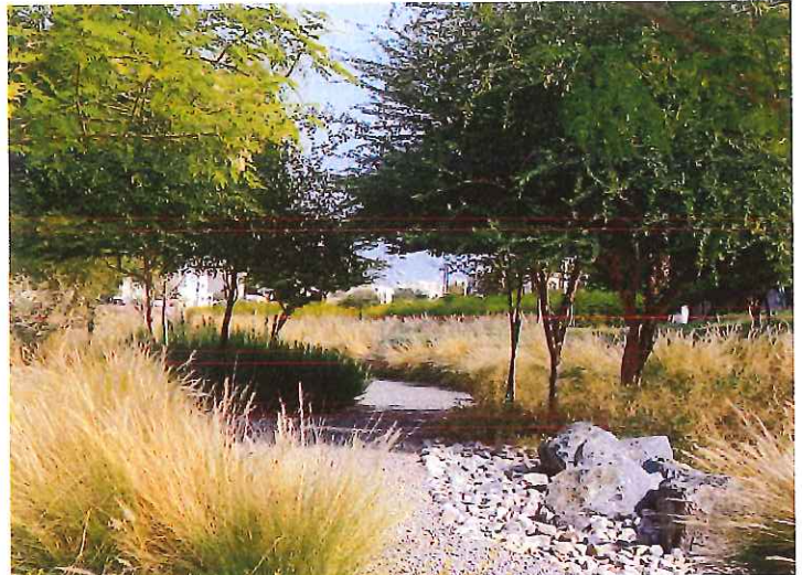
Landscaped stormwater swales can be incorporated as a feature within open space areas
