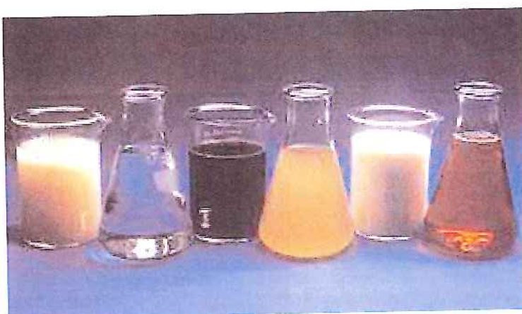
Fig. 6-1. Liquid admixtures, from left to right: antiwashout admixture, shrinkage reducer, water reducer, foaming agent, corrosion inhibitor, and air-entraining admixture. (69795)
