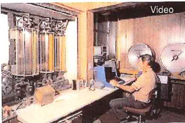
Fig. 6-20. Liquid admixture dispenser at a ready mix plant provides accurate volumetric measurement of admixtures. (44220)
