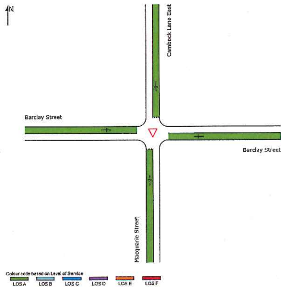
Figure 27: Barclay Street/ Macquarie Street/ Cambock Lane Existing Weekday AM Peak Hour Approach LOS
