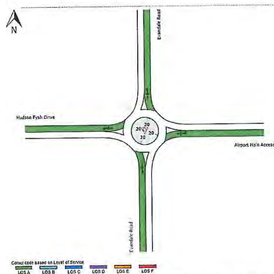
Figure 17: Launceston Airport Entrance/ Hudson Fysh Drive/ Evandale Main Road Roundabout - Existing Operation AM Peak Hour LOS
