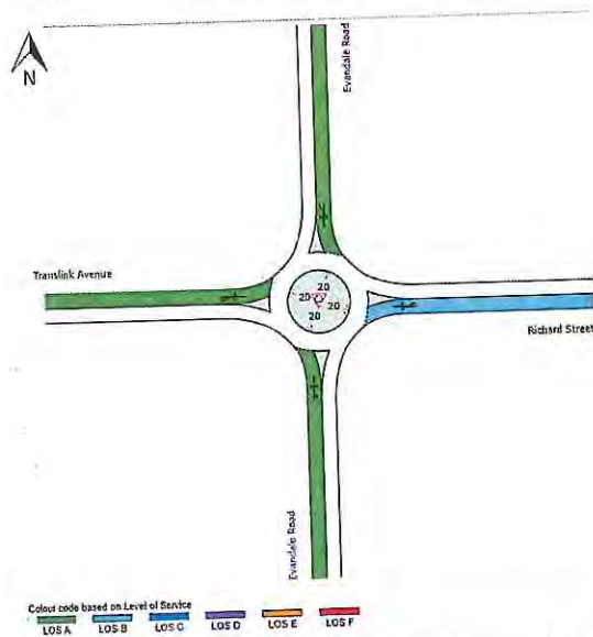
Figure 15: Translink Avenue/ Richard Street/ Evandale Main Road Roundabout - Existing Operation AM Peak Hour LOS
