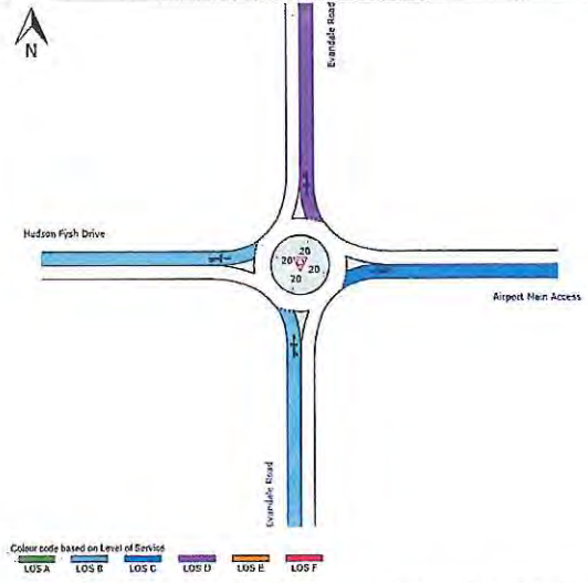
Figure 30: Launceston Airport Entrance/ Hudson Fysh Drive/ Evandale Main Road Existing Roundabout - 2021 Operation PM Peak Hour LOS
