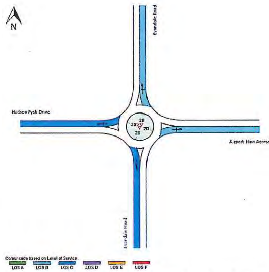
Figure 31: Launceston Airport Entrance/ Hudson Fysh Drive/ Evandale Main Road Existing Roundabout - Operation 2031 AM Peak Hour LOS
