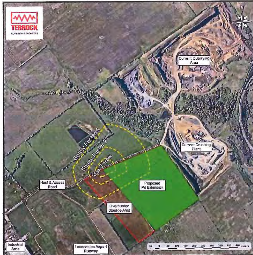
Figure 2 – Flyrock model for closet potential blasting to the TasWater catchment
