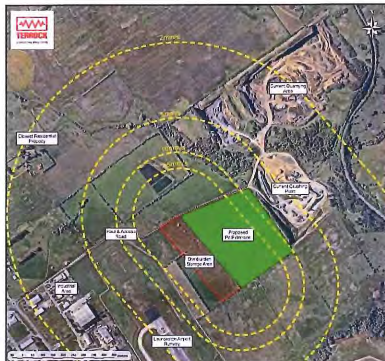
Figure 1 – Ground vibration overlay based on blasting work authority limit
