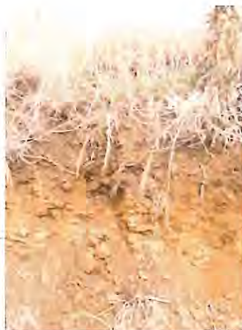
Photograph 5 : Typical soil profile - depth of topsoil at between 150-300 mm
