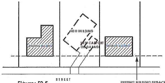
Figure: F2.5 INAPPROPRIATE BUILDING ORIENTATION
