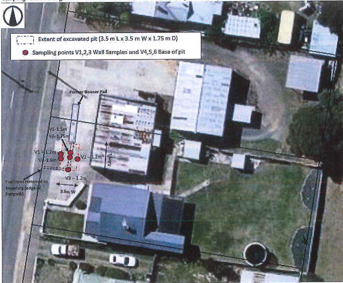
Figure 25: removal of Fuel Lines to the South of former bowser pad.
