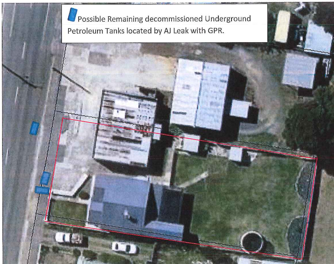
Figure 22: Location of Possible Remaining Underground Fuel Tanks
