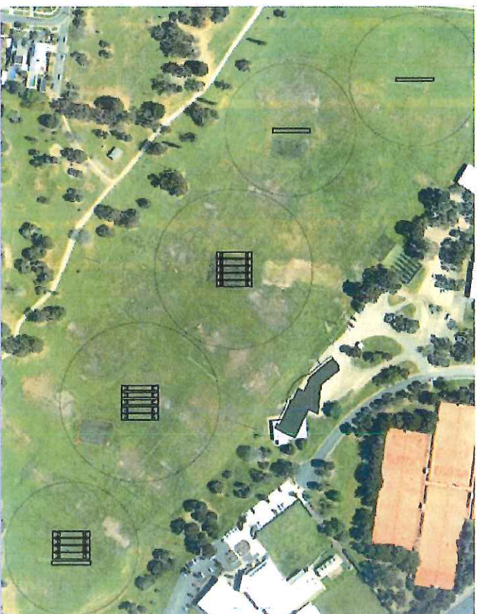
Example of multiple north-south orientated playing field Image courtesy of InsideEDGE Sport and Leisure Planning
