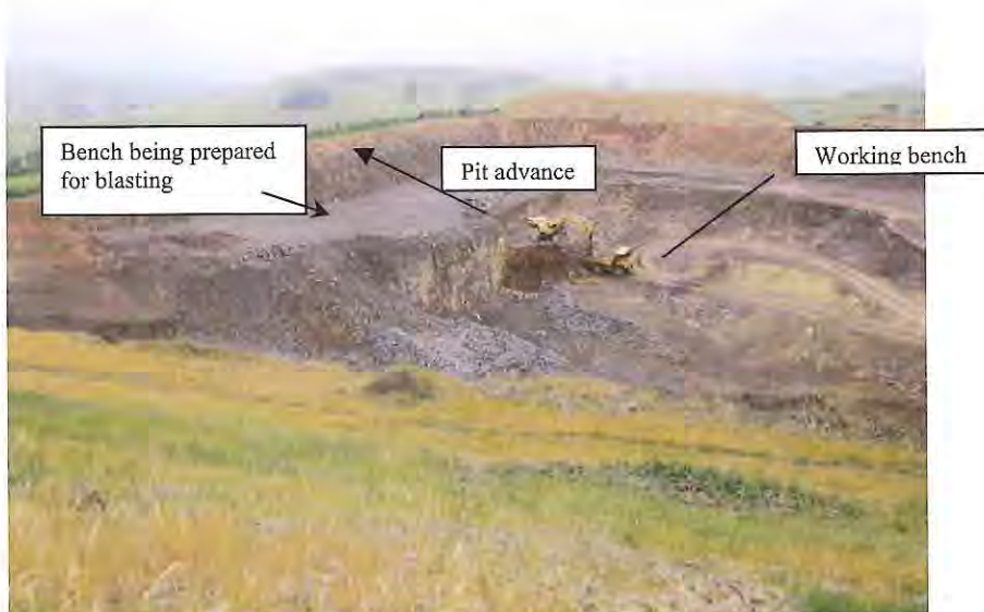
Photograph 1: Typical quarry bench operation. Quarry advances to the left
