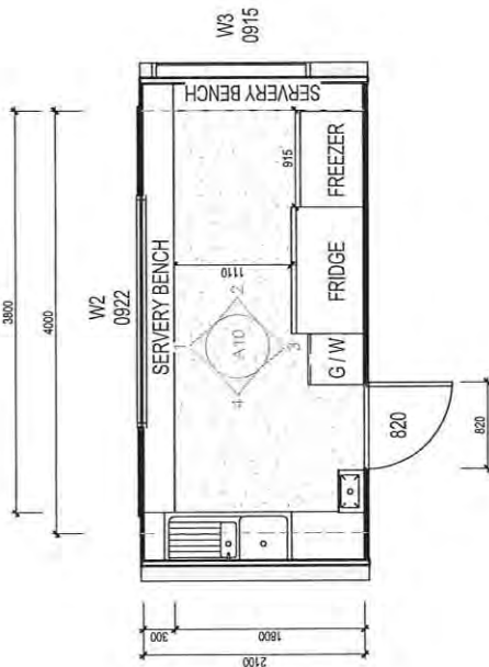
CARAVAN BAR FLOOR PLAN SCALE 1 : 50
