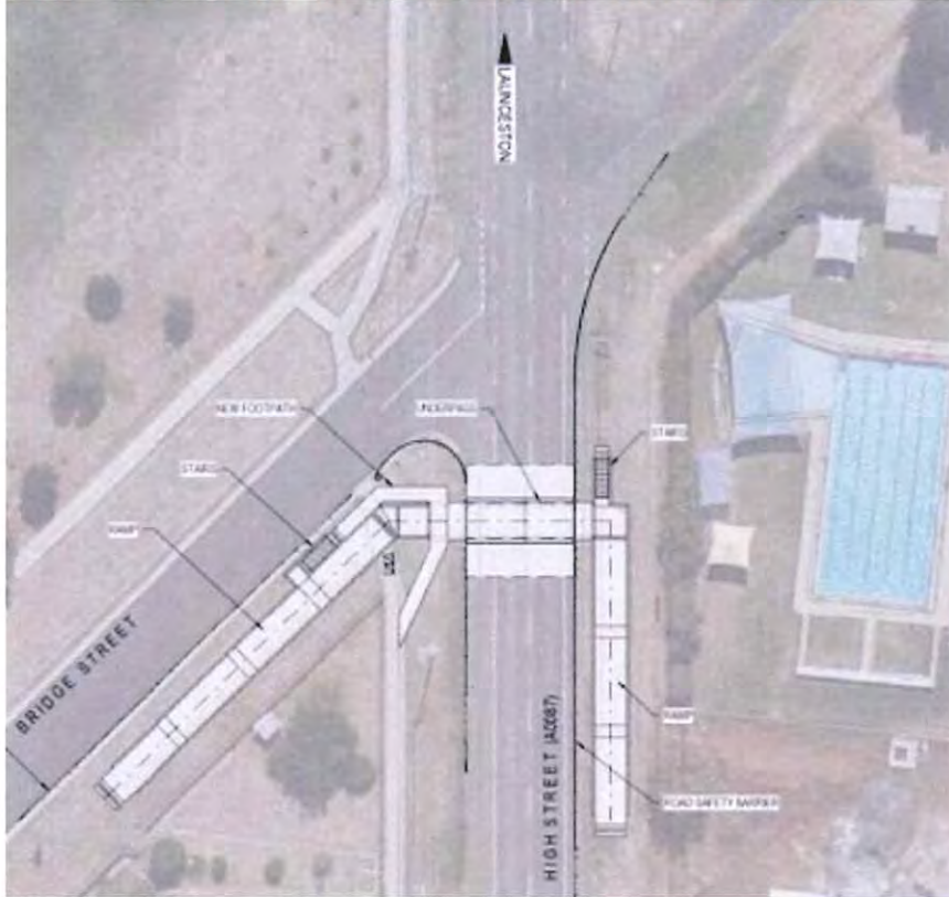
Figure 9 – Anticipated High Street / Bridge Street intersection layout
