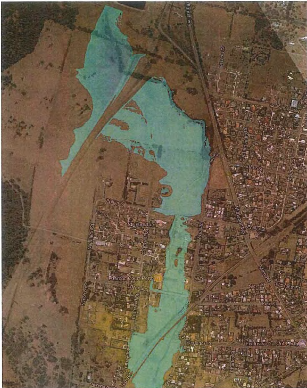
Figure 3 - SDF of 200ML dam with Highway
