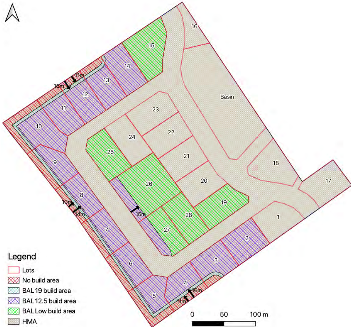
Figure 4-2: BAL construction areas
