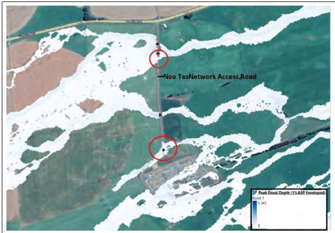
Figure 3: Areas that are subject to shallow overland flow (0.1 to 0.2m) during a 1% AEP event
