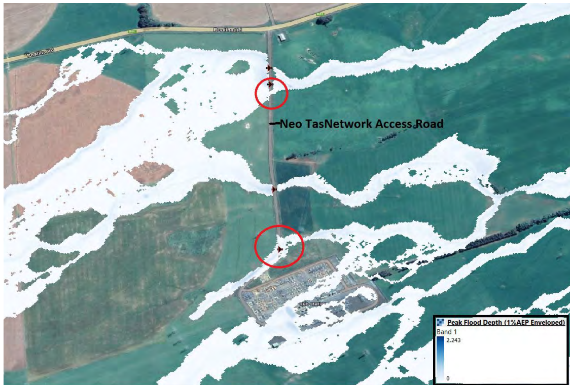
Diagram 7: The existing access road was overtopped in 1% AEP design event (shown in red circle).
