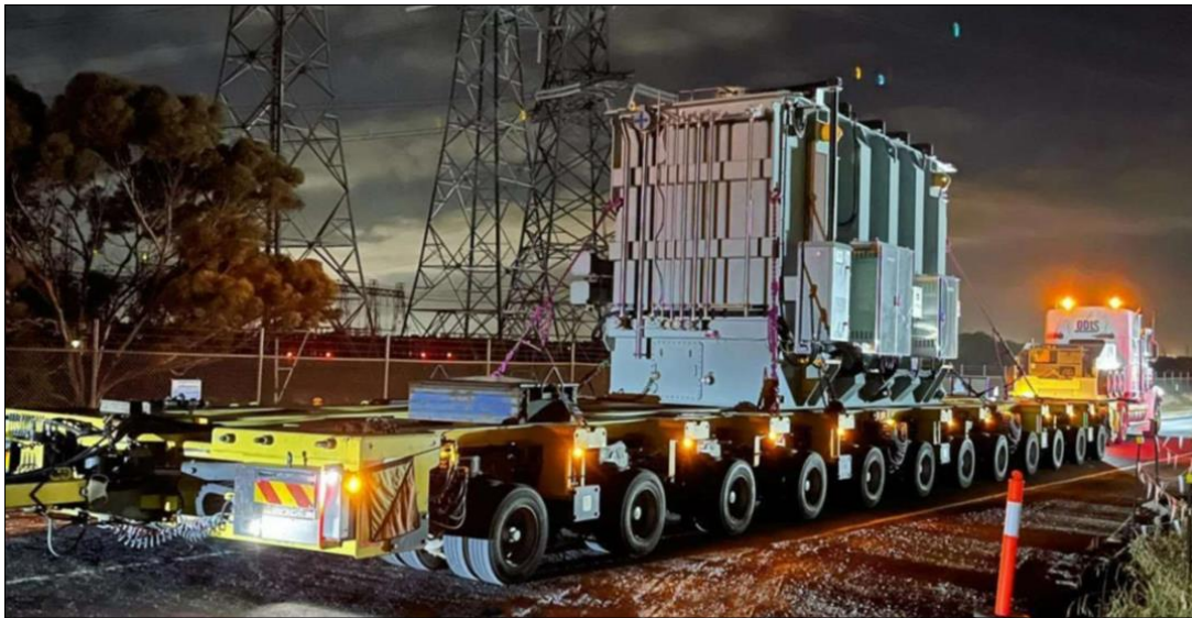
Figure 8: Large power transformer transporter
