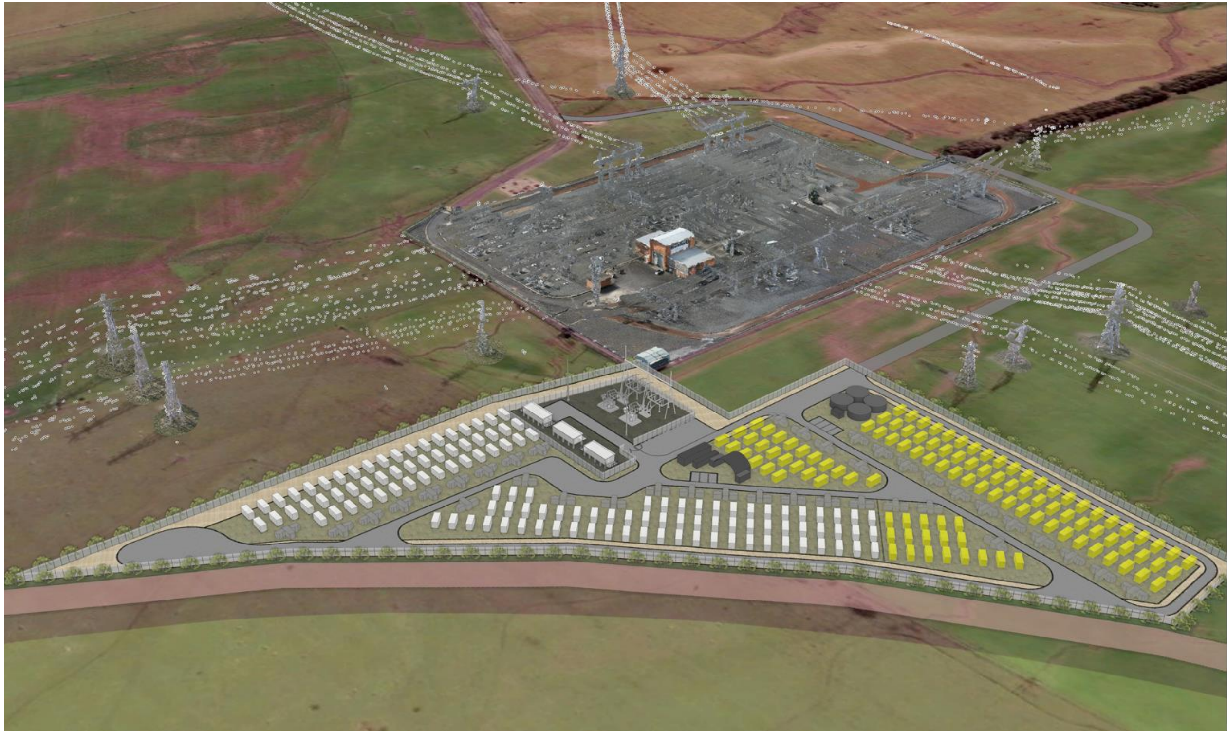
Figure 10: 3D model of the layout. The battery units for Stage 1 are shown in white, the units for Stage 2 are shown in yellow.
