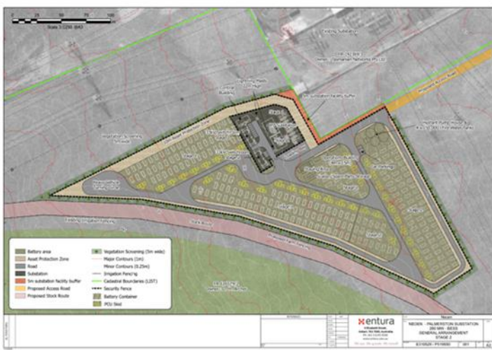
Figure 3: Site Layout of the battery storage location.
