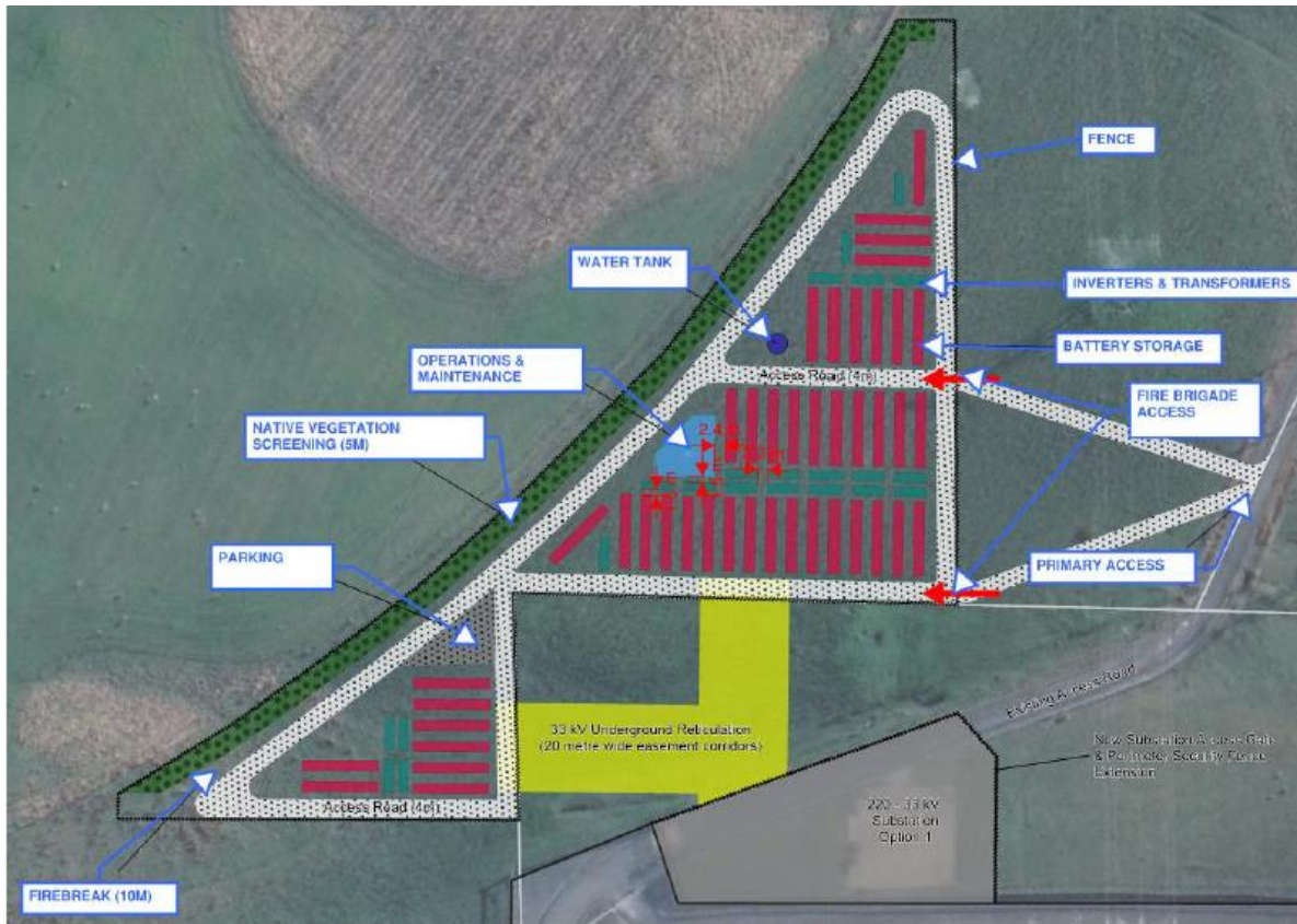
Figure 13 Concept plan - Main site access - Extract Fire Hazard and Risk Assessment, Palmerston BESS (Battery Energy Storage System) NJM Design July 2023 Figure 12 at p.20
