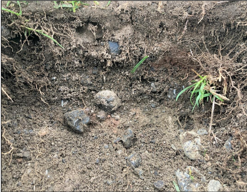
Image 3. Eastfield SPC soil profile 2 on foothills of Class 6 land. Shallow (approx. 10cm), black sandy loam overlying light grey fine sand subsurface on compacted clay. Presence of stones and ironstone nodules throughout profile (taken at site assessment on 29/04/22).
