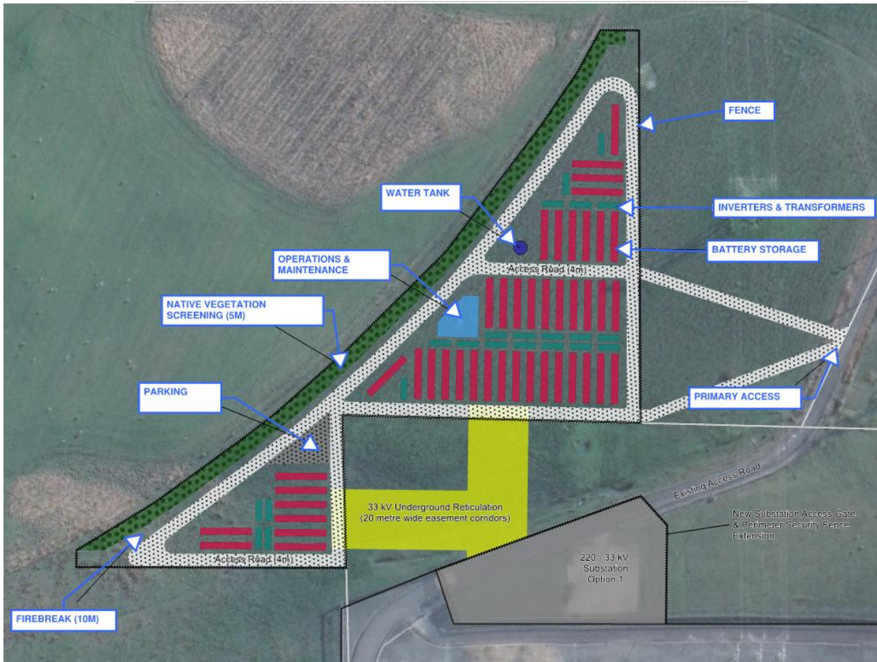
Figure 10 - BESS array layout
