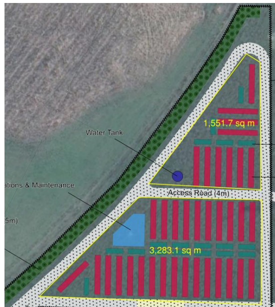
Figure 33: Arrays of battery Storage units.
