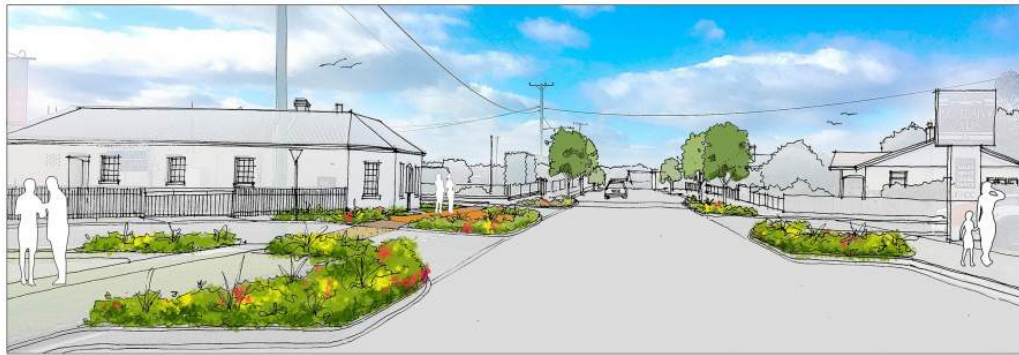
Artist Impression - Main Street and Fairlough Street intersection kerb build-outs with planting.
