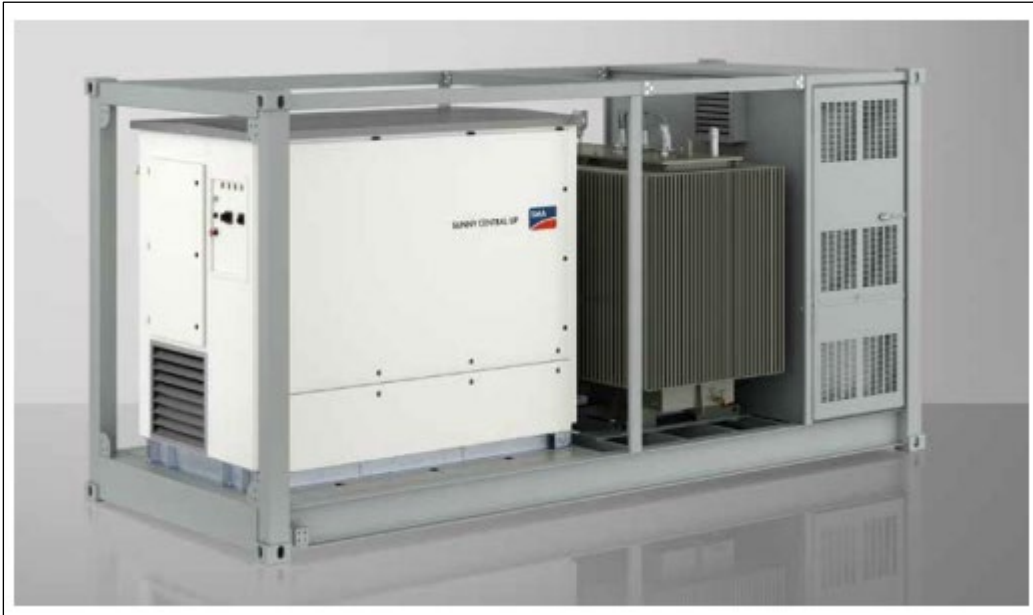
Figure 6: typical inverter/PCU. The inverters facilitate the conversion of direct current (DC) from the solar arrays into alternating current (AC). They are spaced throughout the solar array and are approximately 6 m long, 2.9 m high and 2.4 m wide. (source: Cogency ibid)
