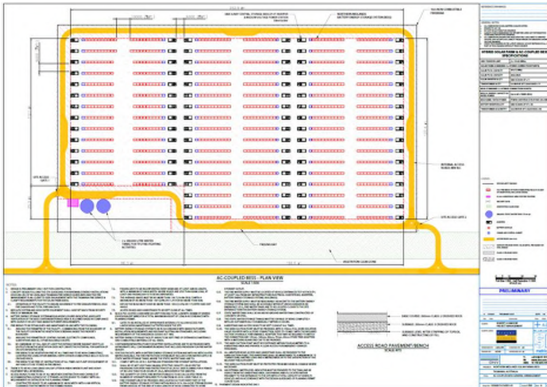
Figure 4: Site specific BESS layout.
