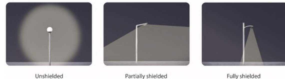
Figure 11 - Light Shielding (Source: Department of Environment and Energy National Light Pollution Guidelines for Wildlife 2020)
