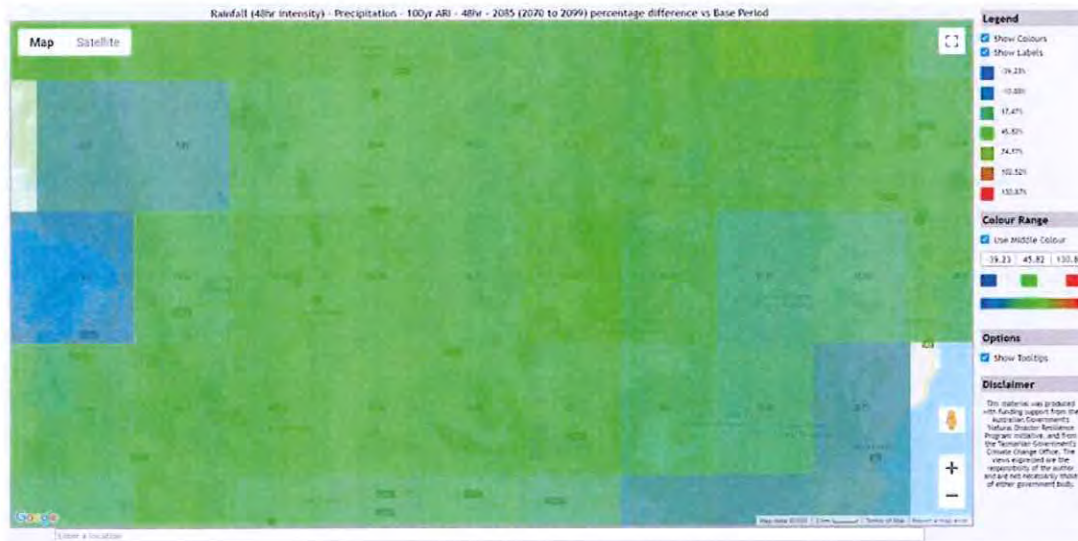
Figure F.2: ClimateAsyst estimates of increase in 1:100 AEP 48 hour duration rainfall intensity
