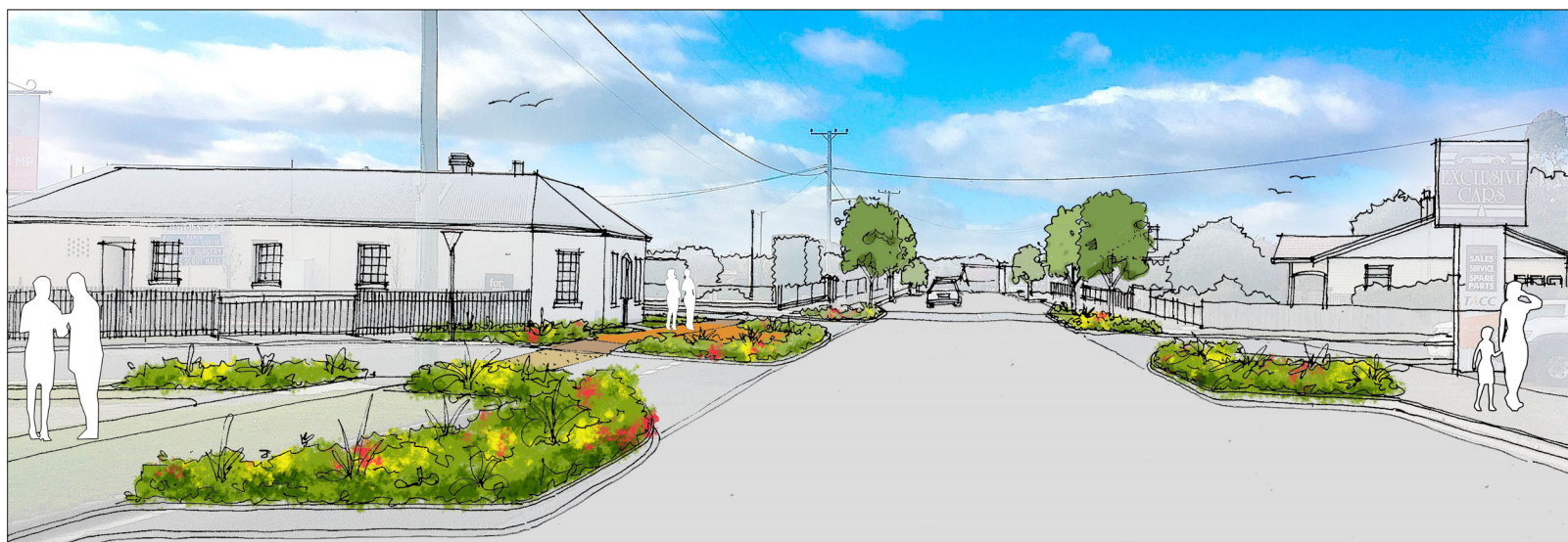
Artist Impression - Main Street and Fairtlough Street intersection kerb build-outs with planting.
